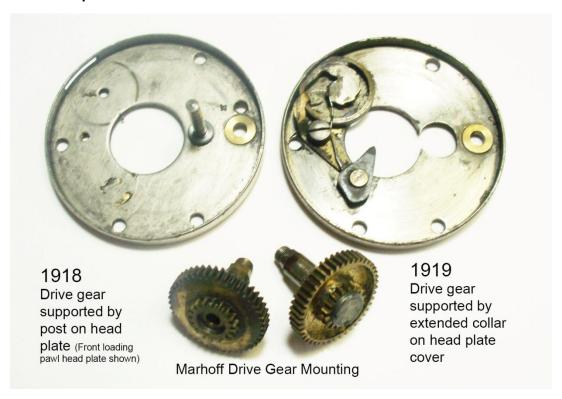
In the first 1919 Model Marhoff, Shakespeare introduced the idea of eliminating the post or spindle used to support the main drive gear, and simply use the drive gear collar on the head plate cover for support. This required adding a brass bushing inside the collar, lengthening the collar, lengthening the
